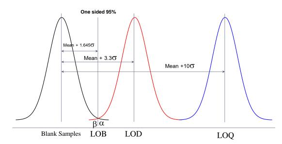
Figure 2: Limit of blank (LOB), limit of detection (LOD), and limit of quantitation (LOQ) based on the blank.
